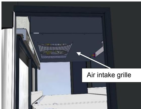
Fig. 2: Air intake grille
